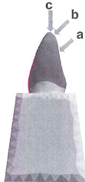
Fig. 3 Direction of the occlusal force a : Loading for the center of the lingual surface of the crown at 45° b : Loading for the incisal edge of the crown at 45° c : Loading for the incisal edge of the crown at 0° to the long axis of the tooth
